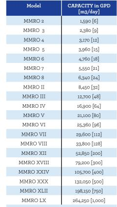
Note: Capacities are based seawater with a TDS of 35,000 ppm at 77°F (25°C).
