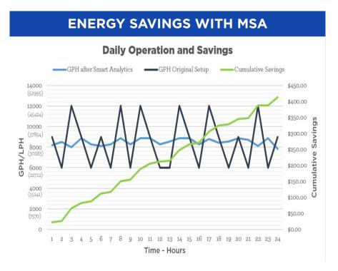
Running all units at fractional load in lieu of starting and stopping to make up demand saves 50 percent on energy with the same total output.
