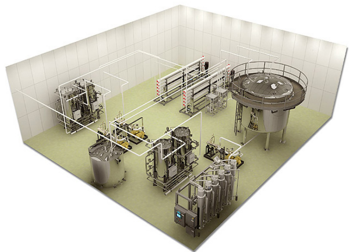
A typical system layout for a multiple-effect-based system using reverse osmosis as pretreatment, with intermediate and final storage and distribution tanks.
