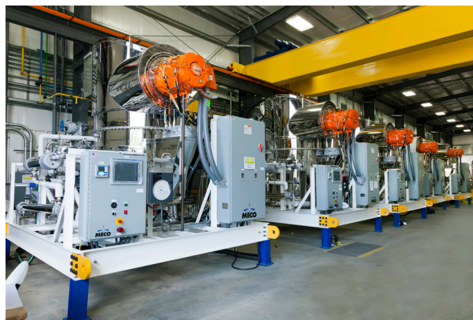
Vapor compression plants for WFI production with high-efficiency sanitary direct drive centrifugal compressors.
